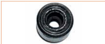
interior ring damaged for 100%
